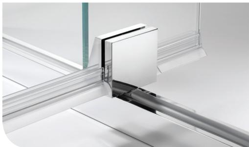
Unique pivot design allows a totally frameless door. Utilising a captive stainless steel top pivot pin, the Vogue 5050 Shower Screen System features a 'positive close' low friction design mechanism, providing the benefit of whisper-quiet and trouble-free operation.
